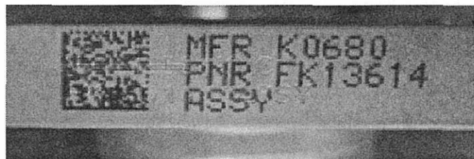
Figure 1: Human readable marking in close proximity to two-dimensional symbol
