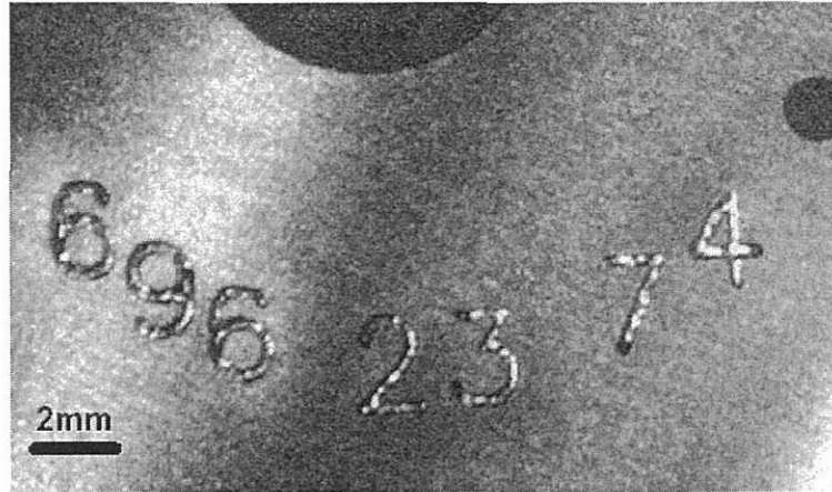
Figure B.7 — Raised lettering using LENS marking
